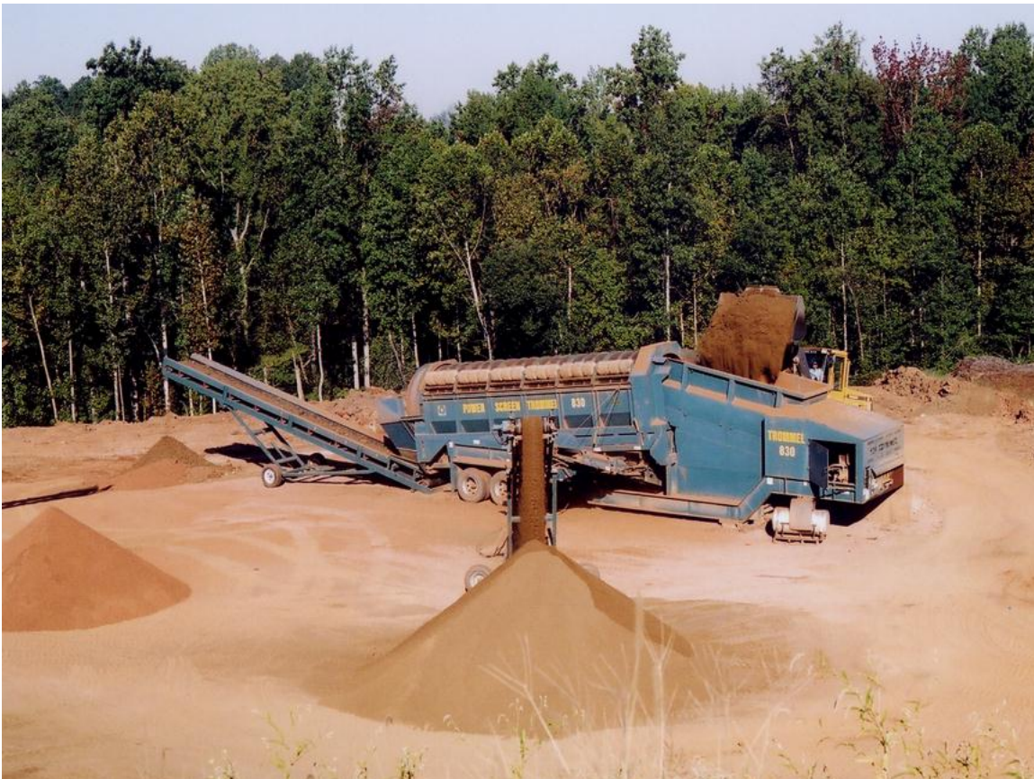
At Blue Max Materials, a screening machine is used to remove debris & break up clumps in soil. Clean soil comes out in one pile & rejected soil full of debris in another.
